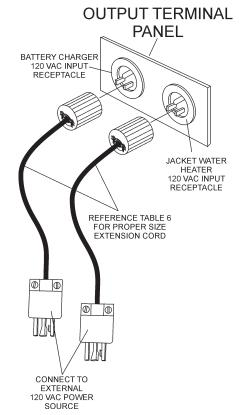
Figure 61. Battery Charger and Jacket Water Heater Power Connections If the generator will be used daily, the battery should normally not require charging. If the generator will be idle (not used) for long periods of time, apply power to the battery charger receptacle via commercial power using a power cord of adequate size.
